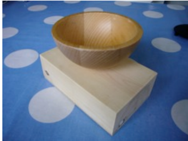
Figure 7: The rapid prototyping of the basic platform: a simple wooden block with a USB interface.
