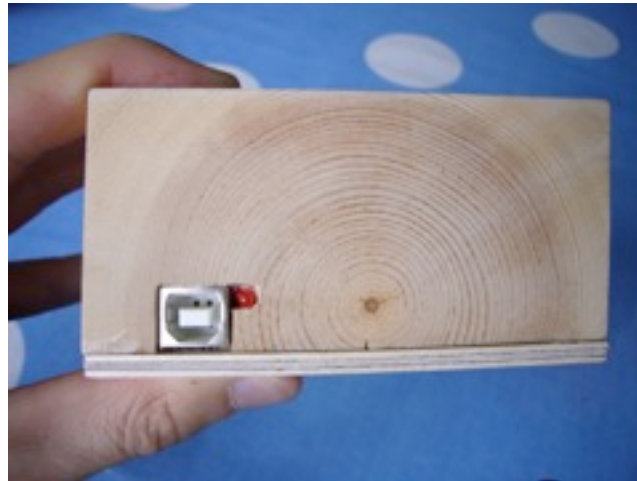
Figure 18. The test-platform is a piece of wood containing an RFID-reader and USB socket.
