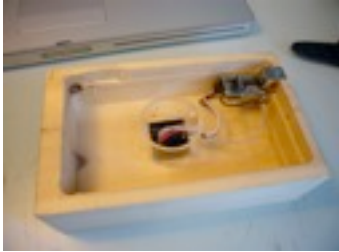
Figure 21. The inside of the prototype-box. An Innovation ID-12 RFID-reader and an usb-adapter.
